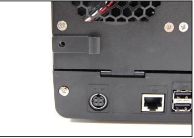
9. <u>Close the back cover and fix it with the four screws.</u>
